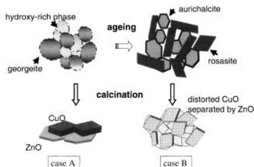
Figure 20. Evolution of microstructural characteristics with ageing of the precursors and the resulting oxides.
